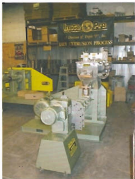
Insta-Pro fish feed extruder with shaped feeds cutter head, aquatic feeds pre-conditioner, and cutter drive
